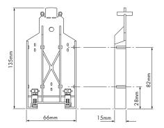
Figure 4.5: IMB57 Insulating mounting block
