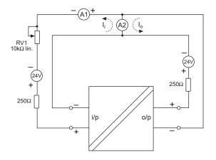
Figure 8.8: AI test circuit #4 "active i/p - o/p sinking"
