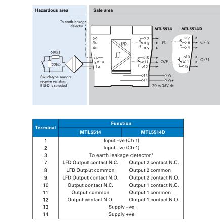
\* See Section 3.1.3 - modules require signal plug HAZ1-3 for access to this function.
