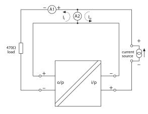
Figure 8.11: AO test circuit
