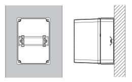
Figure 5.3: Optimum orientation for wall mounted enclosure
