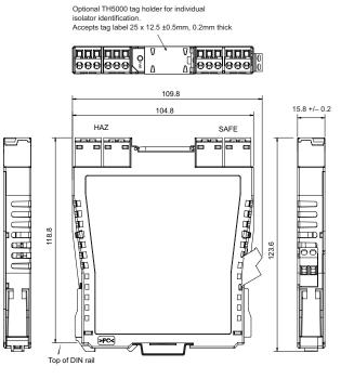
Figure 3.1: Dimensions of MTL5500 package
