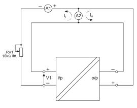
Figure 8.5: AI test circuit #1
