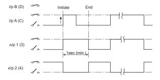
Mode 10: As mode 9 with line fault c/o
