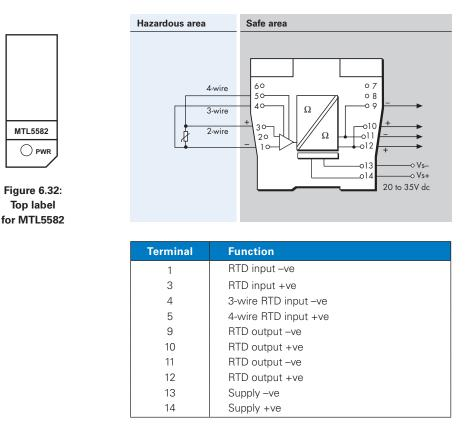
**Warning**: Check polarity of terminals used for safe-area connections. Safe-area terminals 9, 10, 11 and 12 are unipolar so it is essential to select a positive terminal on the MTL5582 for connection to the positive of the RTD input card.
