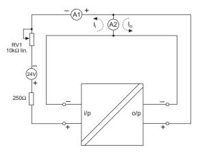
Figure 8.7: AI test circuit #3 "active i/p"
