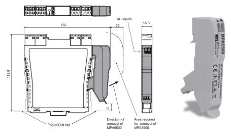
Figure 4.2: MPA5500 AC power adaptor
