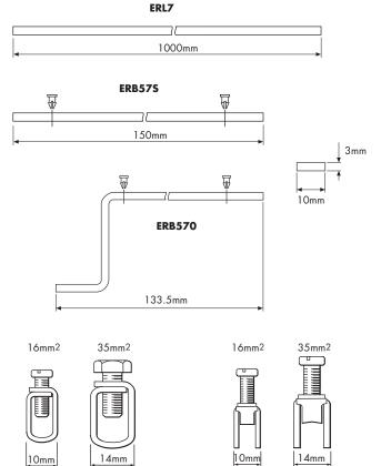
Figure 4.9: Earth rails and clamps
